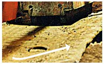
Fig. 2: Deformation of the ladle's steel side plates
