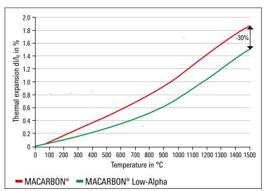
Fig. 3: Reduction of thermal expansion by 30% (integral)
