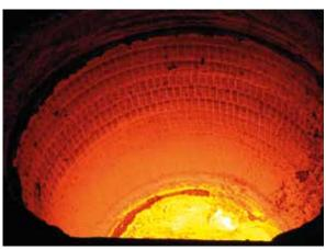
Fig. 5: Field test in a German steelmaking plant: MACARBON® lining with Low-Alpha technology after 50 heats
